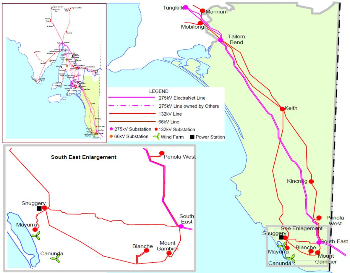
Figure 5-4: South East electricity transmission regions (ElectraNet, 2013)
