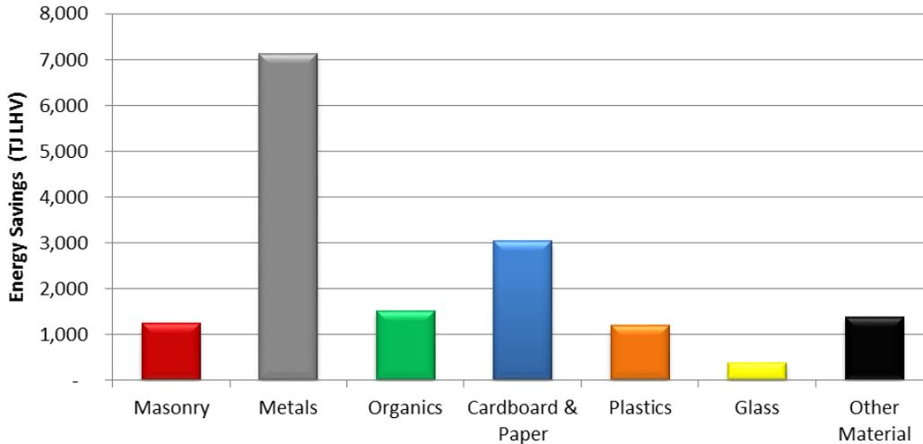
**Figure 7.2** Avoided energy consumption (by material category) as a result of recycling in SA, 2012-13
