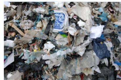
After separating the waste, suppliers to the Kymijärvi II are required to shred it to a particle size of about 6 cm and reduce any moisture content to below 20–30%. A sample from each truckload is tested by a laboratory at the entrance to the power plant’s weigh station. Processed waste is delivered to the plant’s fuel depot.
