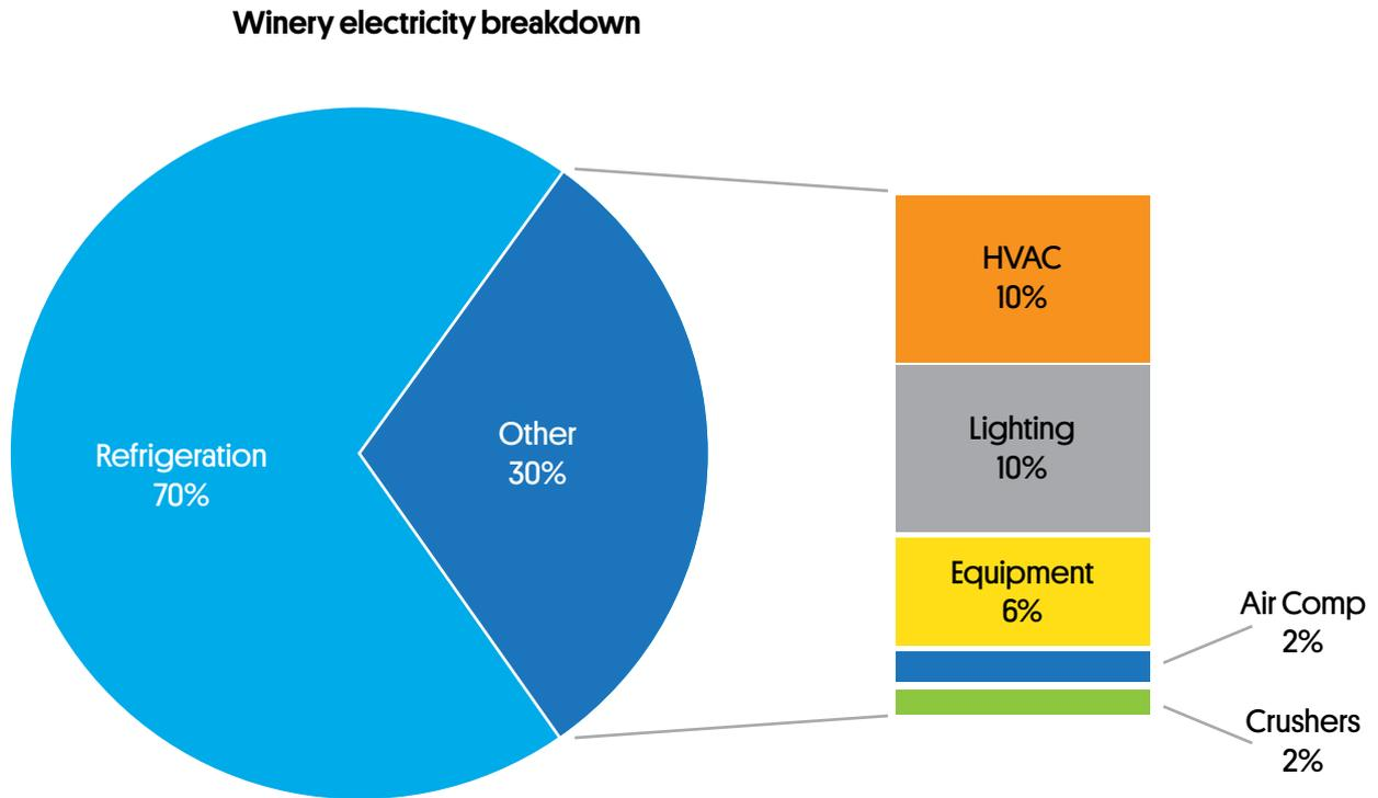
Figure 16: Winery Electricity Use Breakdown
