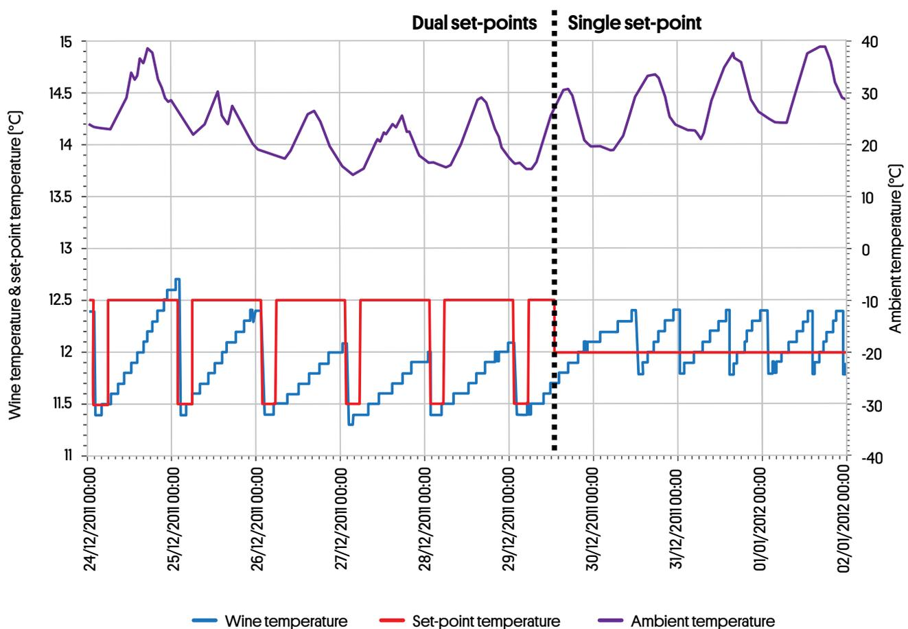
Figure 36: Dual Setpoint Load Shifting
