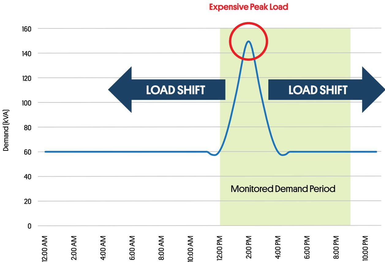
Figure 17: Load shifting
