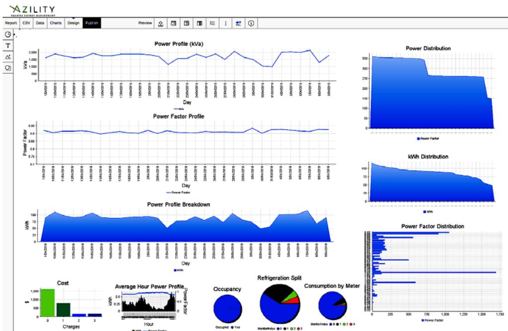
Figure 13: Example of well-presented interval meter data
