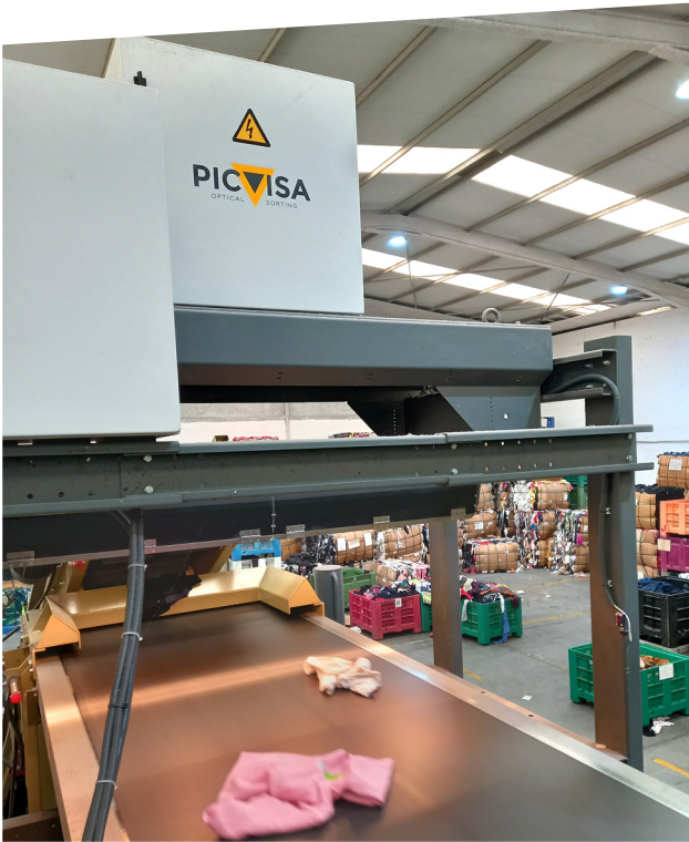
Figure 6: Garments passing along a conveyor belt are identified by composition and color with a mixed system of Artificial Vision and NIR Spectra
