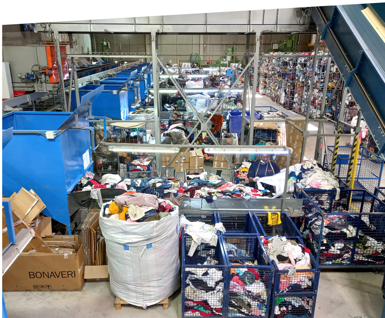
Figure 8: Waste textile items manually sorted for reuse before being sorted by composition at Formació i Treball
