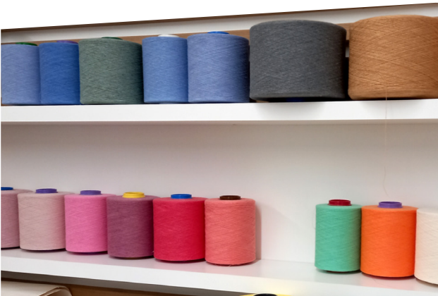
Figure 11: At Valérius 360 waste textiles are colour sorted enabling yarns to be produced without the use of dyes
